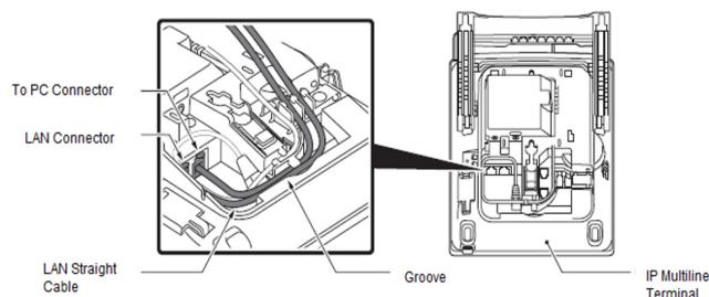
**!** When using the PC port with a local power supply, depending on the LAN cable connector housing, the LAN cable connector may not fit. Remove the outer plastic covering from the LAN cable connector, or use the LAN cable with a thin connector.
